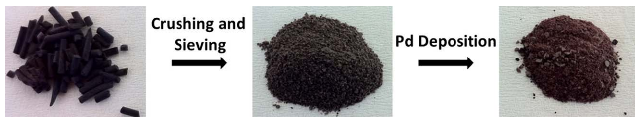
Figure 1. Example of Pd/Au/Al 2 O 3 prepared from Au/Al 2 O 3 pellets (1.2 wt% Au).
